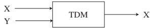
Figure 9 . The Turbo Decoder Module: \mathbf{X} = (X_1, \dots, X_k) , the priors in the form of likelihood ratios; \mathbf{Y} = the channel evidence; \mathbf{X}' = (X'_1, \dots, X'_k) , the “extrinsic” likelihoods:
